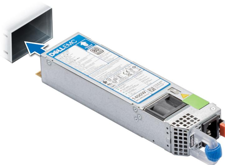
Figure 89. Installing a power supply unit for Front Accessed configuration
