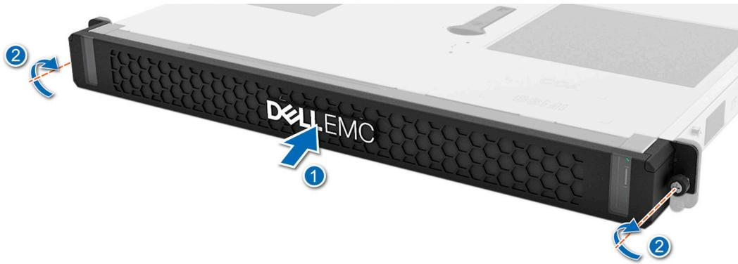
Figure 16. Installing the front bezel for Rear Accessed configuration
