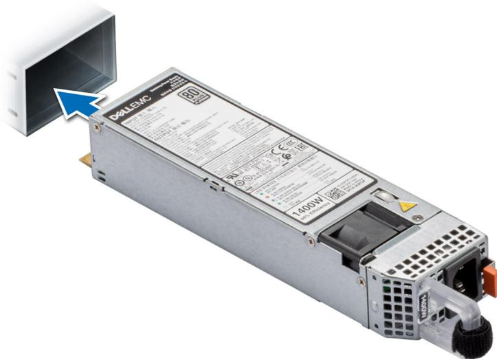
Figure 88. Installing a power supply unit for Rear Accessed configuration
