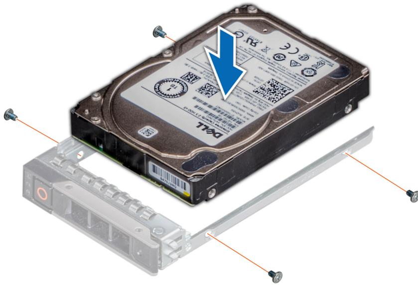
**Figure 36. Installing a drive into the drive carrier**
