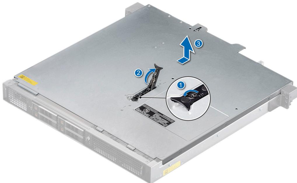
**Figure 20. Removing the system cover for Front Accessed configuration**
