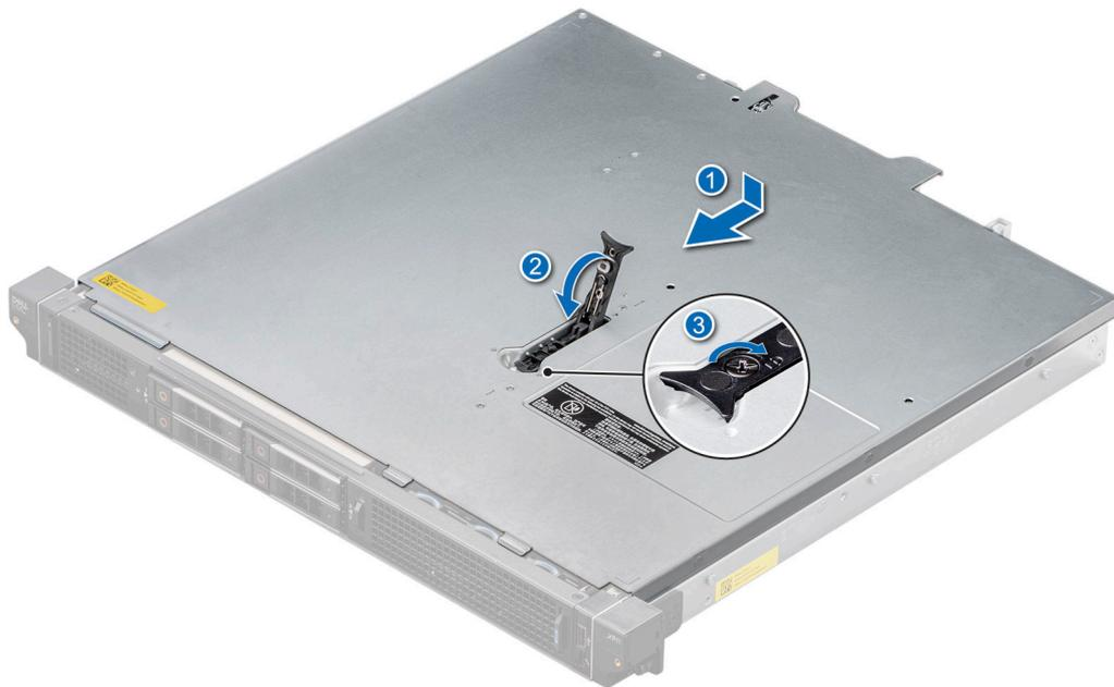
Figure 21. Installing the system cover for Rear Accessed configuration
